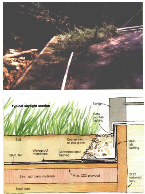
with big gobs of silicone caulk covering both the brackets and the screws. Finally, we place a narrow band of coarse sand or pea gravel along the edge of the 2x4 and around skylights and chimneys to promote quick runoff.
