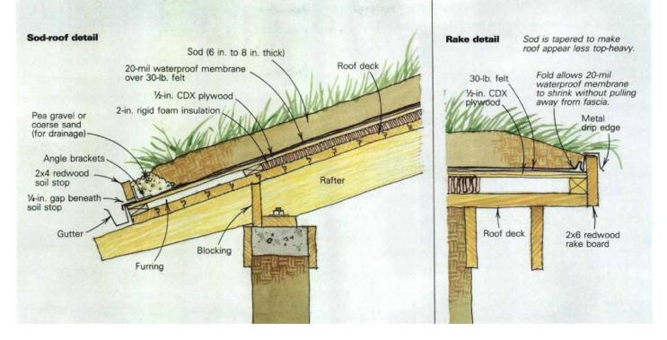
**Roof-top anatomy**–My state-of-the-art sod roof consists of (from bottom to top) the rafters and decking, 2-in. rigid-foam panels, <sup>3</sup>/<sub>8</sub>-in. or <sup>1</sup>/<sub>2</sub>-in. CDX plywood, a layer of 30-lb. felt, a 20-mil or thicker waterproof membrane, and 6-in. to 8-in. of soil (drawings above). I substitute furring strips for the insulation on the overhangs. A narrow band of gravel or sand promotes drainage along the eaves and around chimneys and skylights.
